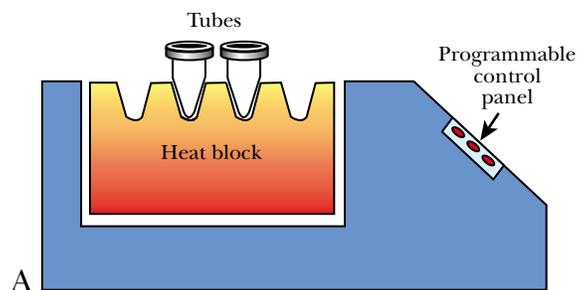
**FIGURE 23.02 PCR Machine or Thermocycler**
