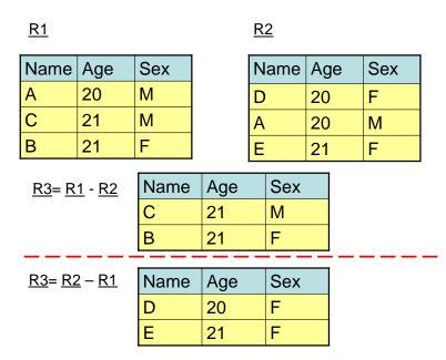
Figure 2.7 – Example of a DIFFERENCE operation on two relations: R1 and R2
