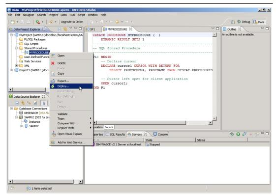
Figure 6.4 – Deploying a stored procedure
