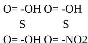
The latter may be regarded as derived from the former by the substitution of the nitro group ( $\text{NO}_2$ ) for the hydroxyl group ( $\text{OH}$ ).
