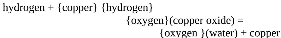
The water formed collects in the cold portions of the tube *C* near its end. In this experiment the copper oxide is said to undergo reduction. *Reduction may therefore be defined as the process of withdrawing oxygen from a compound.*
